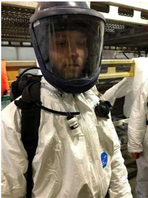
Figure 22: Filters mounted in the insulators breathing zone
