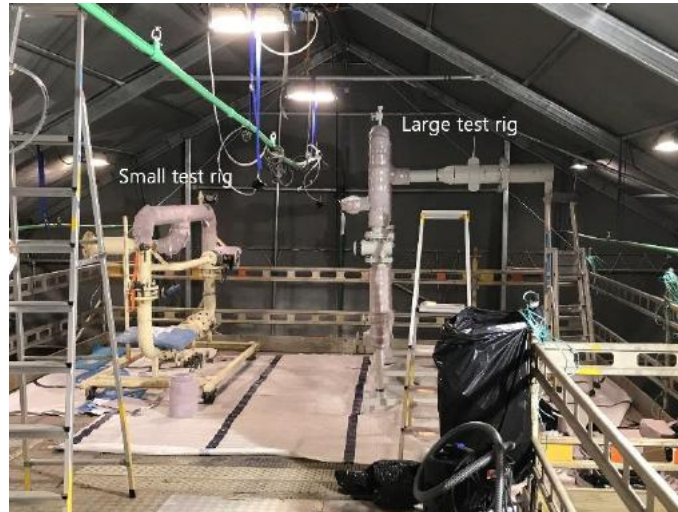
Figure 7: Large test rig and small test rig and their location on the scaffolding work level
