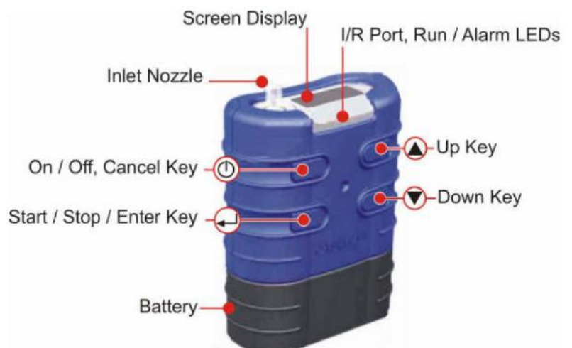
Figure 13: Casella Tuff pump with indication of functions
