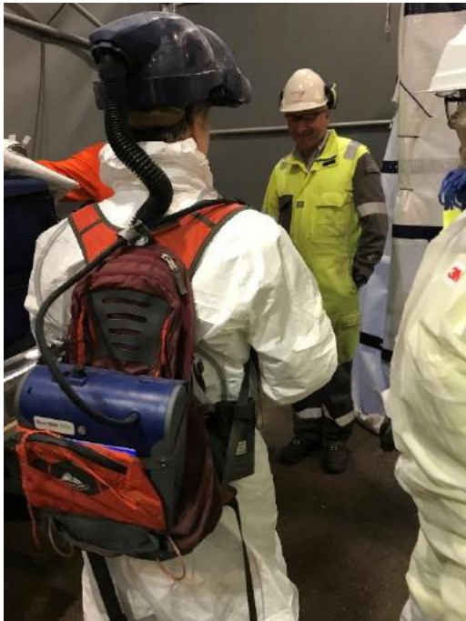
Figure 29: Insulator with DustTrak DRX sampling
