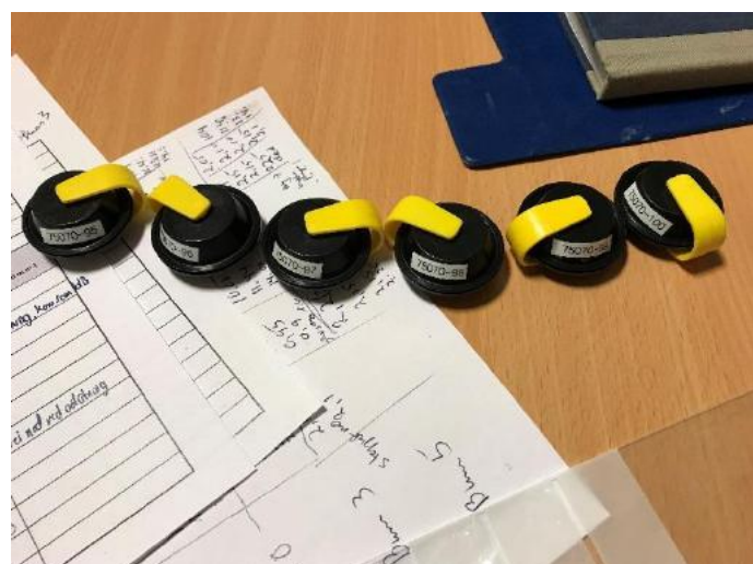
Figure 10: Respirable filter cassettes (inside the sampling head during sampling)
