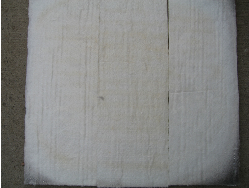
Photo 1 – Exposed Surface of the Inner Layer After 96 hours at 649°C
